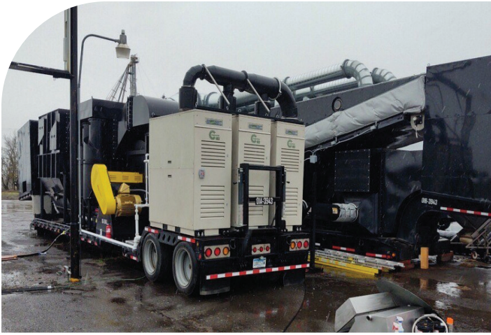
Three propane-fueled Capstone C65 microturbines provide prime power to the mobile drying unit developed by Northwest Agricultural Drying.
